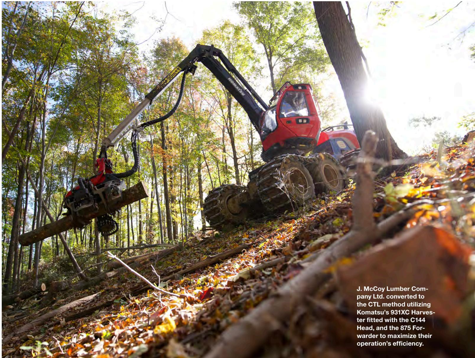
J. McCoy Lumber Company Ltd. converted to the CTL method utilizing Komatsu's 931XC Harvester fitted with the C144 Head, and the 875 Forwarder to maximize their operation's efficiency.
